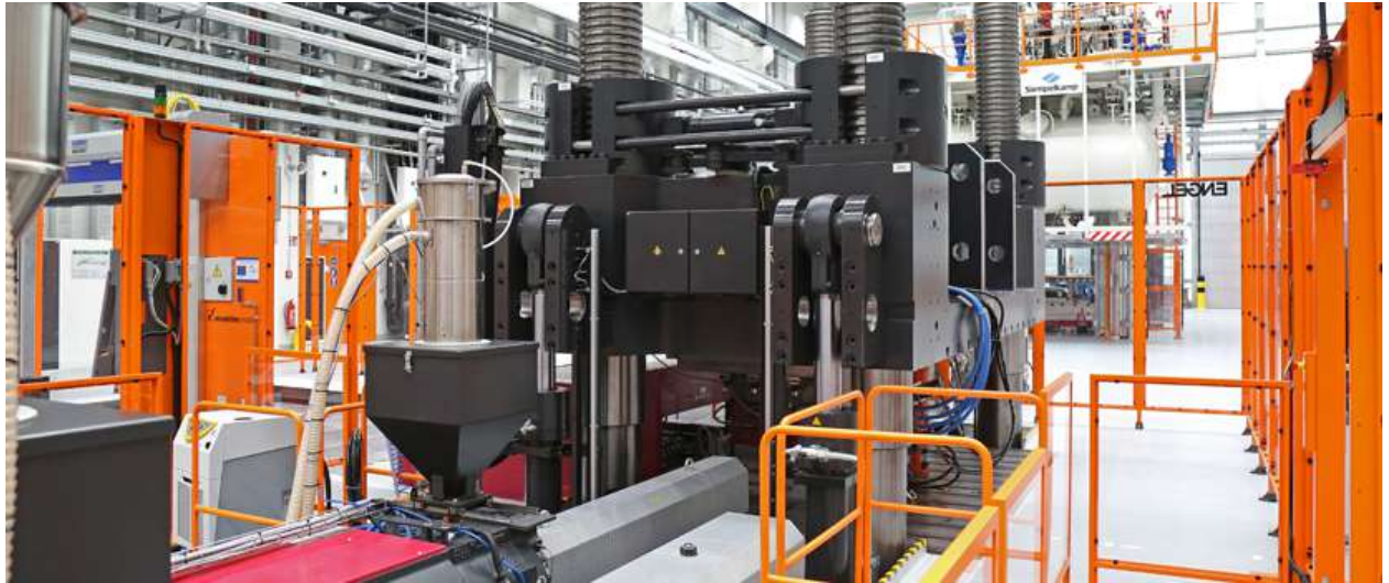
Figure 10: ENGEL v-duo 3600 injection moulding machine
