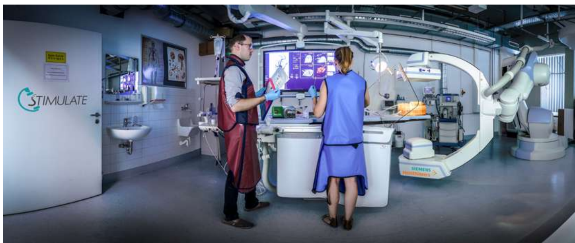
Figure 11: Siemens Artis zeego robot-mounted flat-panel C-arm X-ray system in STIMULATE 's angiography laboratory.
